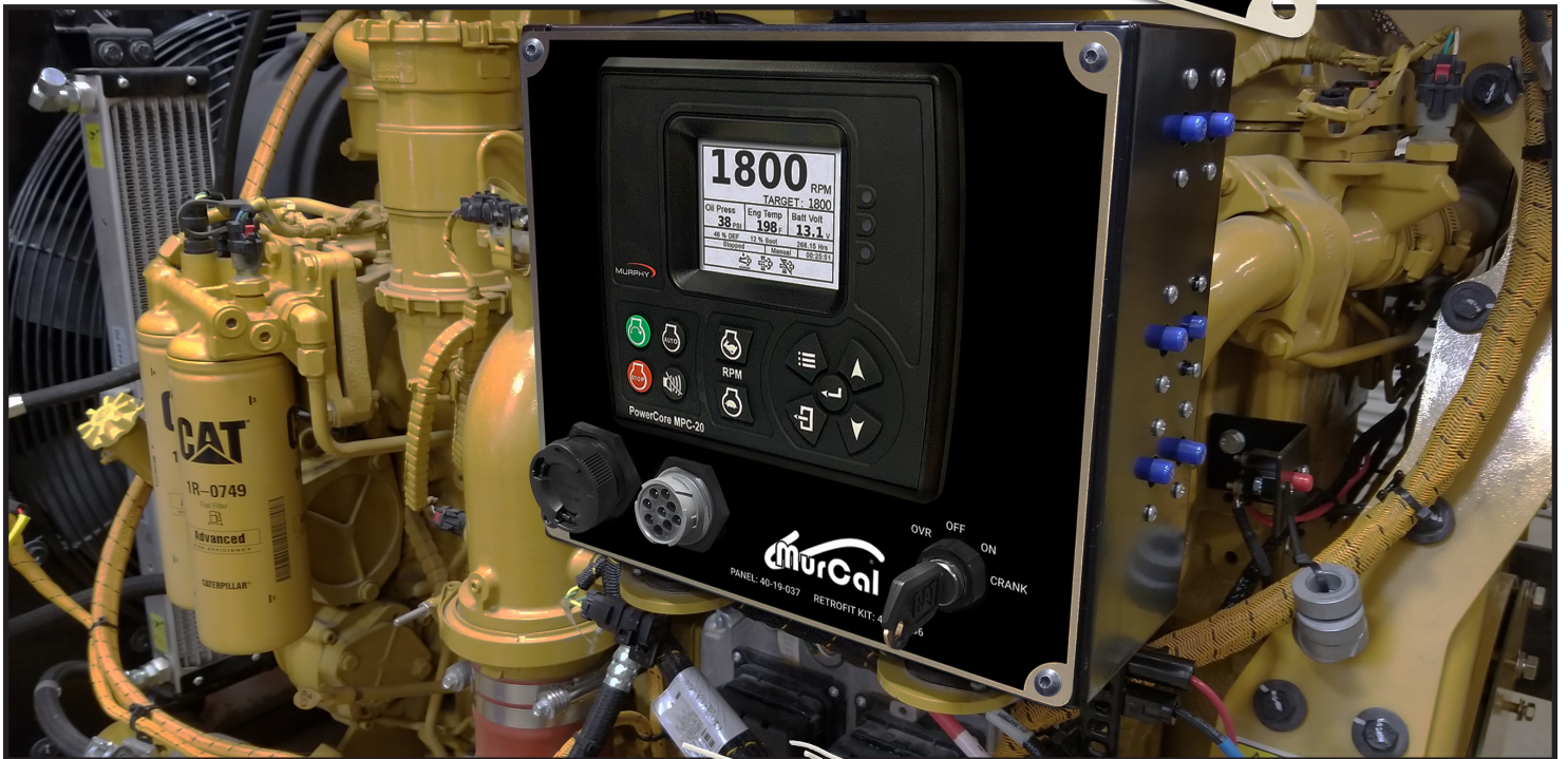
PANEL MOUNTED ON A CAT ENGINE
